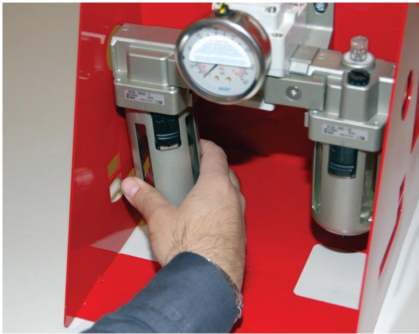
Figure 17. FRL Unit – Lubricator 2/3rds Full of Oil
