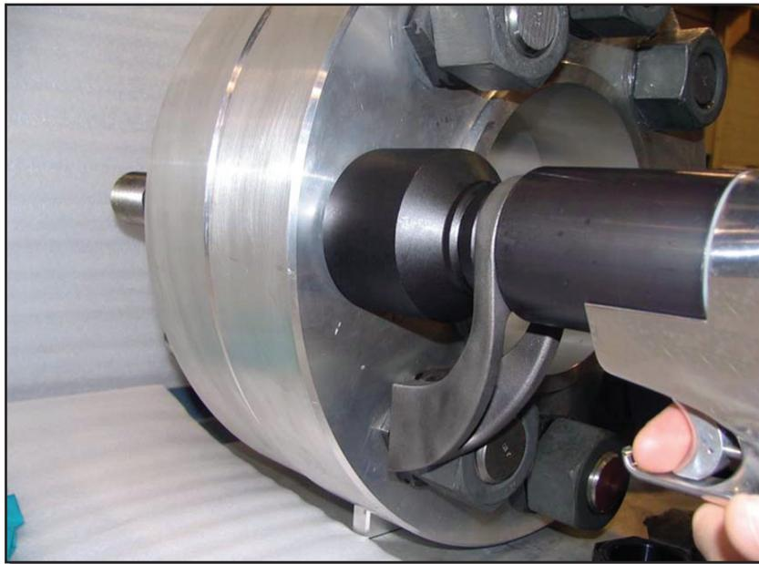
7. Torque the fastener by depressing the trigger until socket stops turning and air bypasses the motor.
