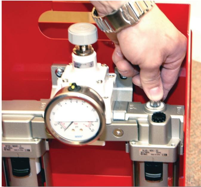
3. Turn the flow adjustment knob clockwise or counter-clockwise until the oil is dripping at a rate of at least one drop every ten seconds.
